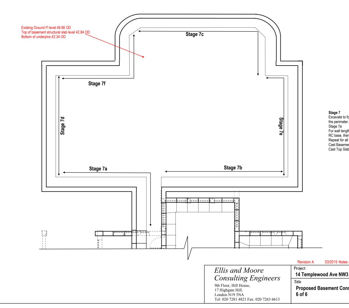
**Stage 7** Excavate to formation level , battering back the perimeter. Stage 7a For wall length, from shuttering and construct RC base, then construct RC wall . Repeat for all stages. Cast Basement Slab Cast Top Slab
