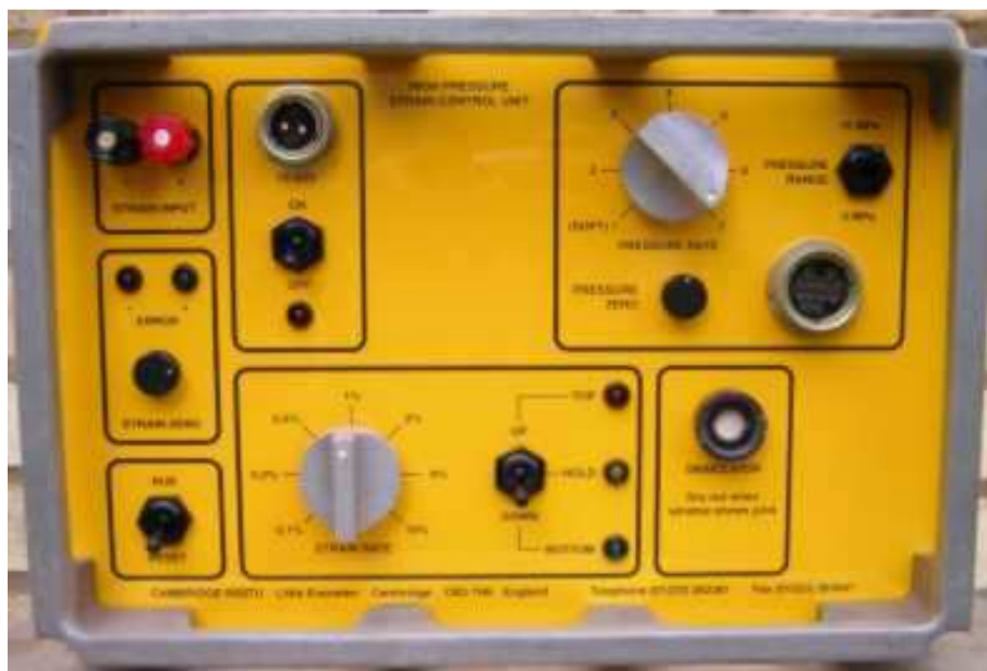
Figure A.5 The Strain Control Unit
