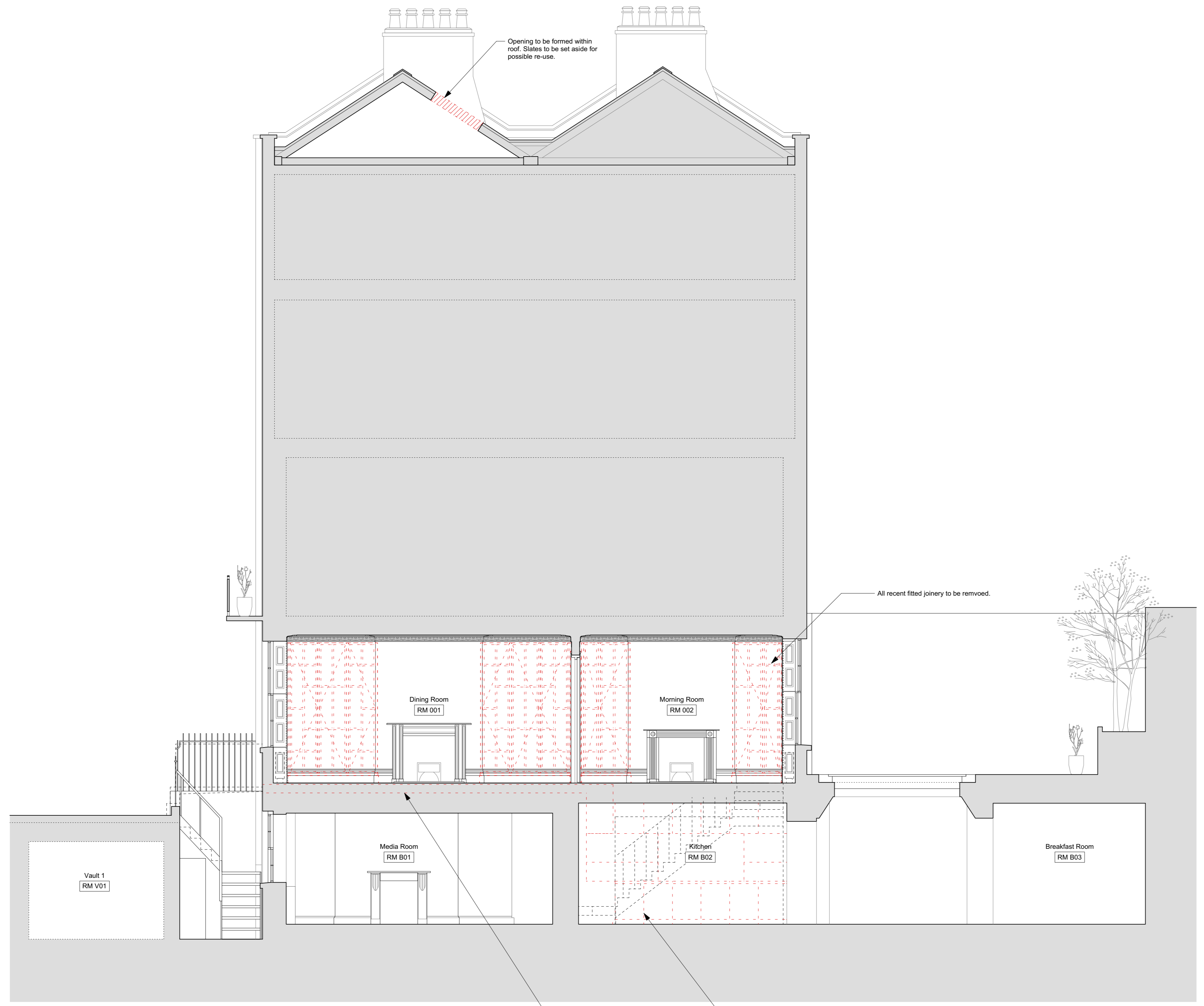
1 Section showing demolition DM-02 Scale: 1:50
