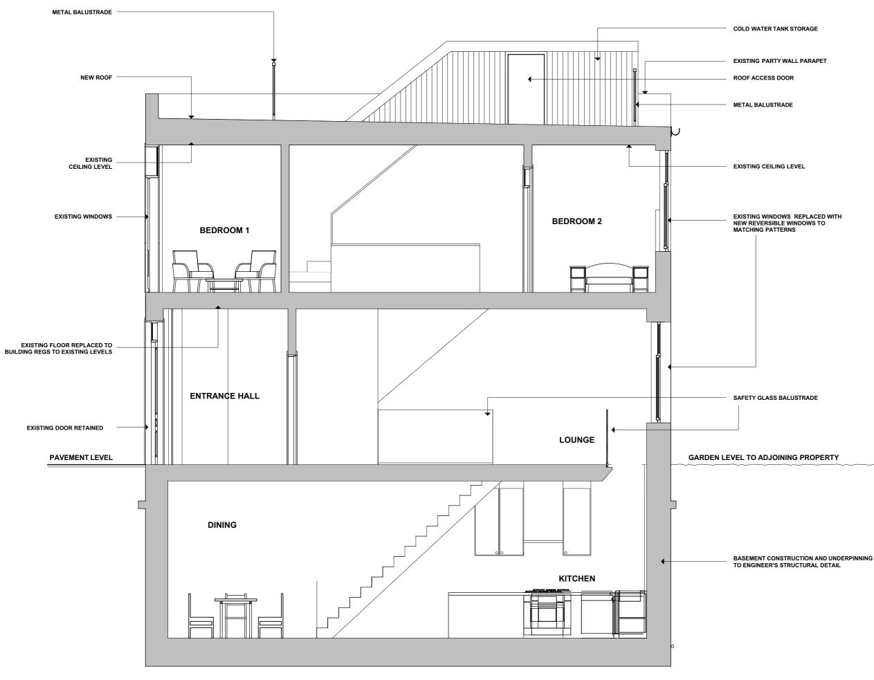
D - 30/04/2015 Adjust roof balustrade C - 21/04/2015 Relocate CWS Tank and adjust glass balustrade. B - 04/02/2015 Reduced height of staircase enclosure at roof level and \_relocation of CWS. A - 19/11/2014 Updated to include retention of facade walls etc. Revisions Scale Metre Scale n. by 1:50 @ A3 СТ 29/09/2014 Drawing PROPOSED SECTION AA Proiec REDEVELOPMENT 61 BAYHAM PLACE, NW1 0ET MODERN CITY ESTATES FLAT 7A, 22 CRAVEN HILL, W2 3DS Drg. No 1767-P-05 D UNIT 306 MARE STREET STUDIOS,
