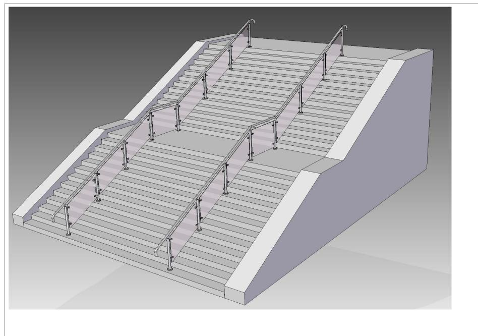
$50 \phi$  316 grade satin polished stainless steel 10mm clear toughened glass infill 0.74KN Loading
