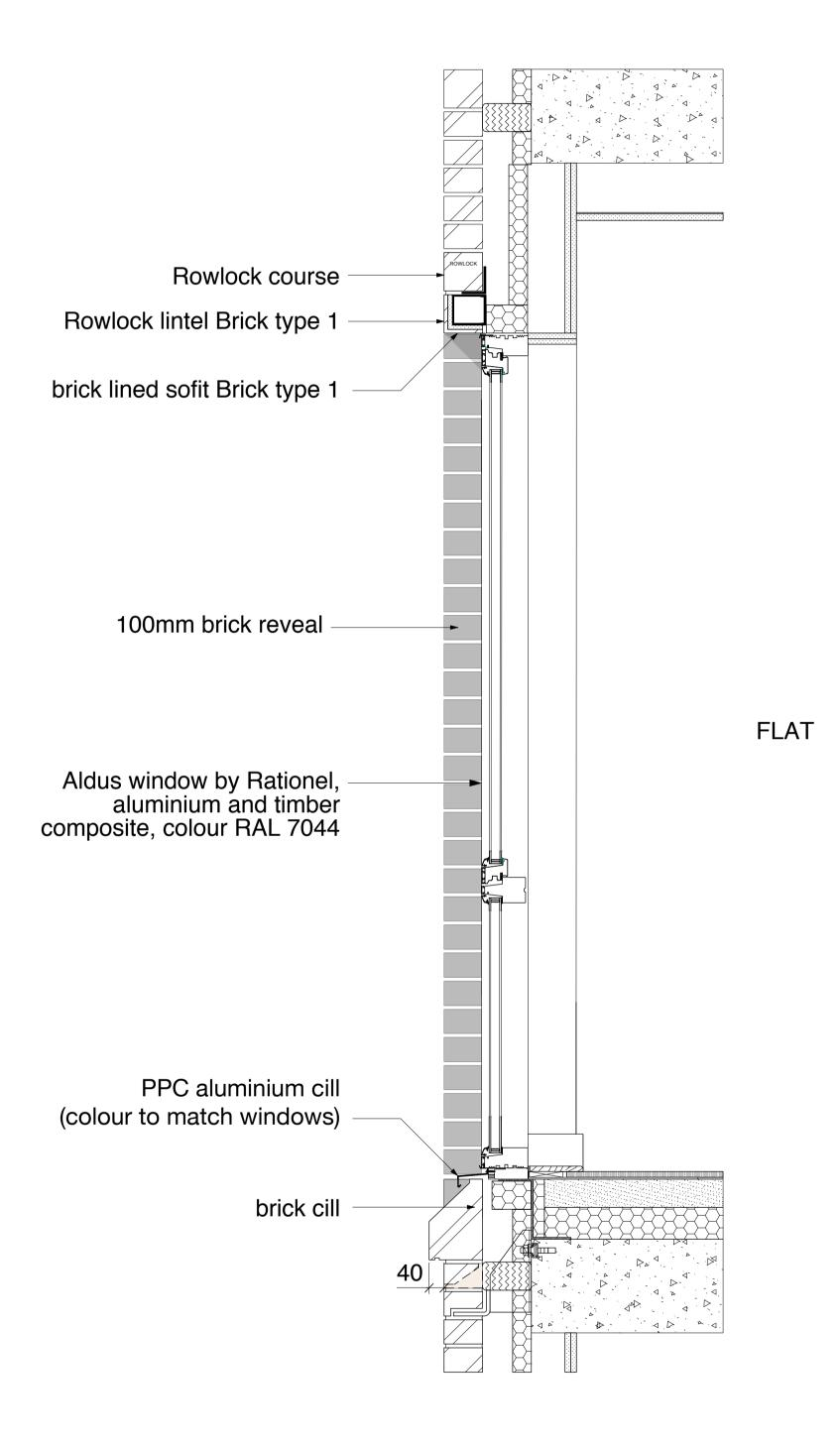
02 TYPICAL WINDOW SECTION WITHIN BRICK TYPE 5 1:10 @A1 / 1:20 @A3
