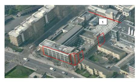
A protective scaffold will be erected to the areas indicated, the scaffolding contractor will have a design and drawings for all scaffold and will also supply all method/risk assessments for the works. The scaffold to Area 1 will be fitted with monoflex acoustic barrier between the occupied building and the building for demolition.
