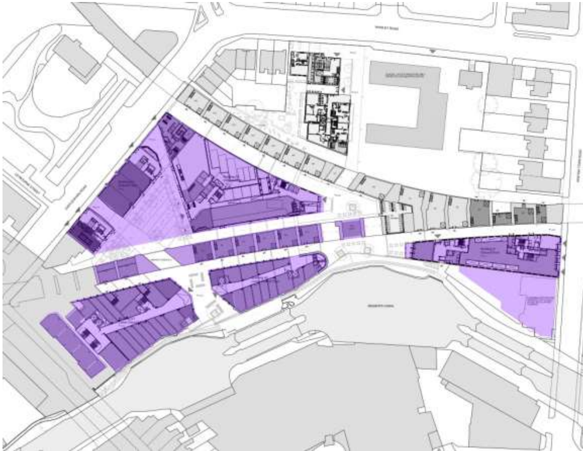
Fig.4: Plan of the application area with proposed single / upper basements highlighted. The northernmost triangular shaped area will have a secondary basement below, but its' location is not deemed archaeologically significant enough to warrant further mitigation
