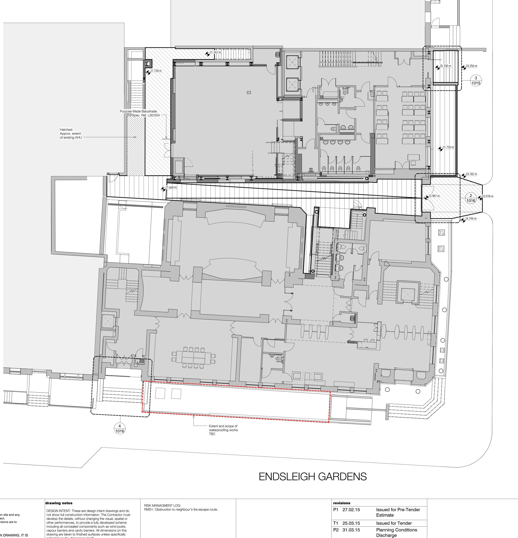
KEY York stone paving Spec: Q25/111 Railing and stone upstand Spec: L30/551 Reconfigure existing slab to Structural Engineer's information
