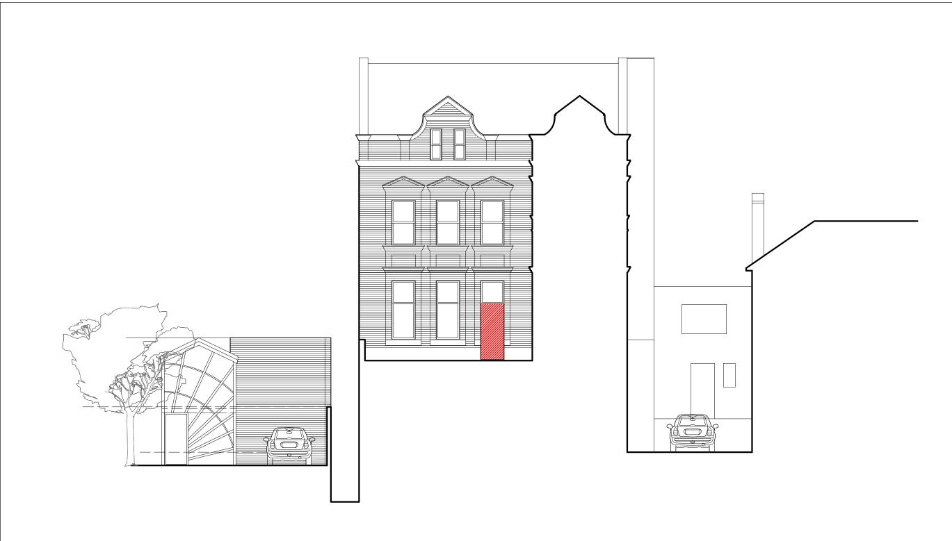
Extent of demolition: Opening made full height Removal of sash window
