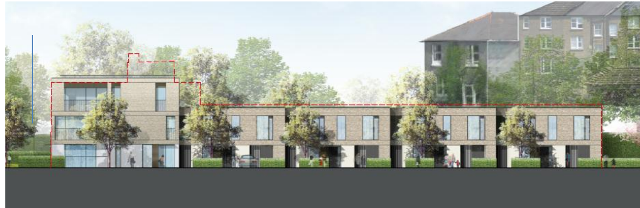
Extract from PRP Architect's Elevation AA4437/2135 - Red Line indicates existing Clubhouse Roof Profile
