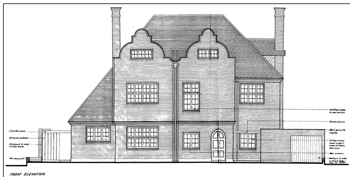
Fig.9 – Original Gable Form Pre-1961 – Source Reference: Ref: TP/10124/22179, dated 25.01.1961
