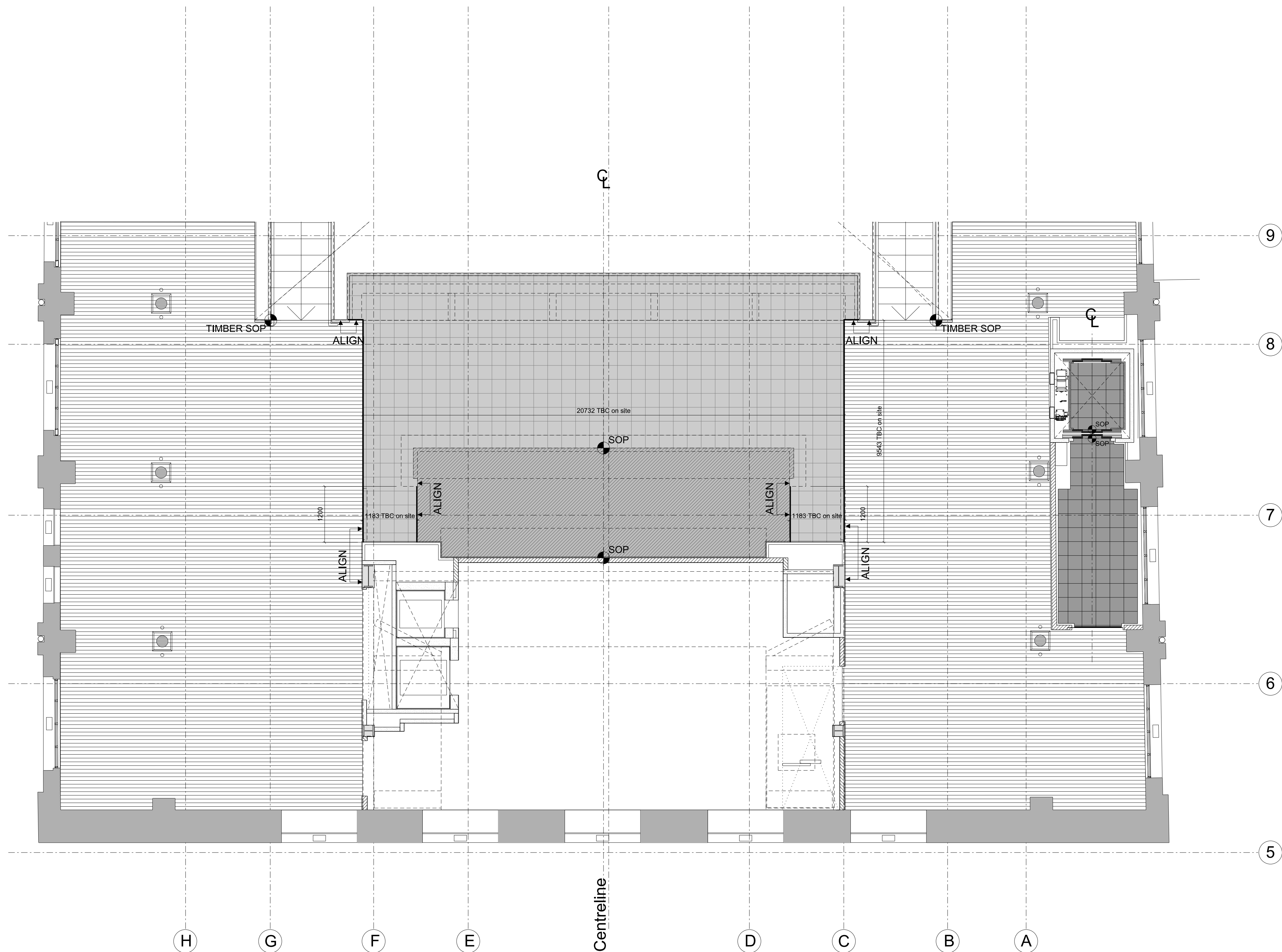
1 GROUND FLOOR Proposed Ground Floor Plan - Marble Setting Out 1:50
