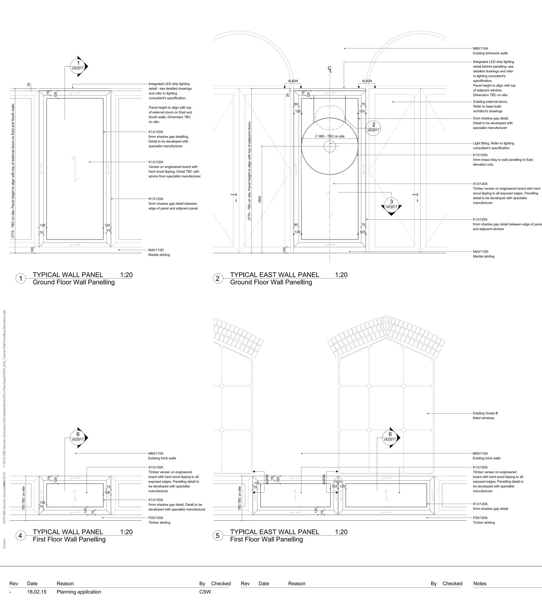
5mm shadow gap detail between edge of panel
