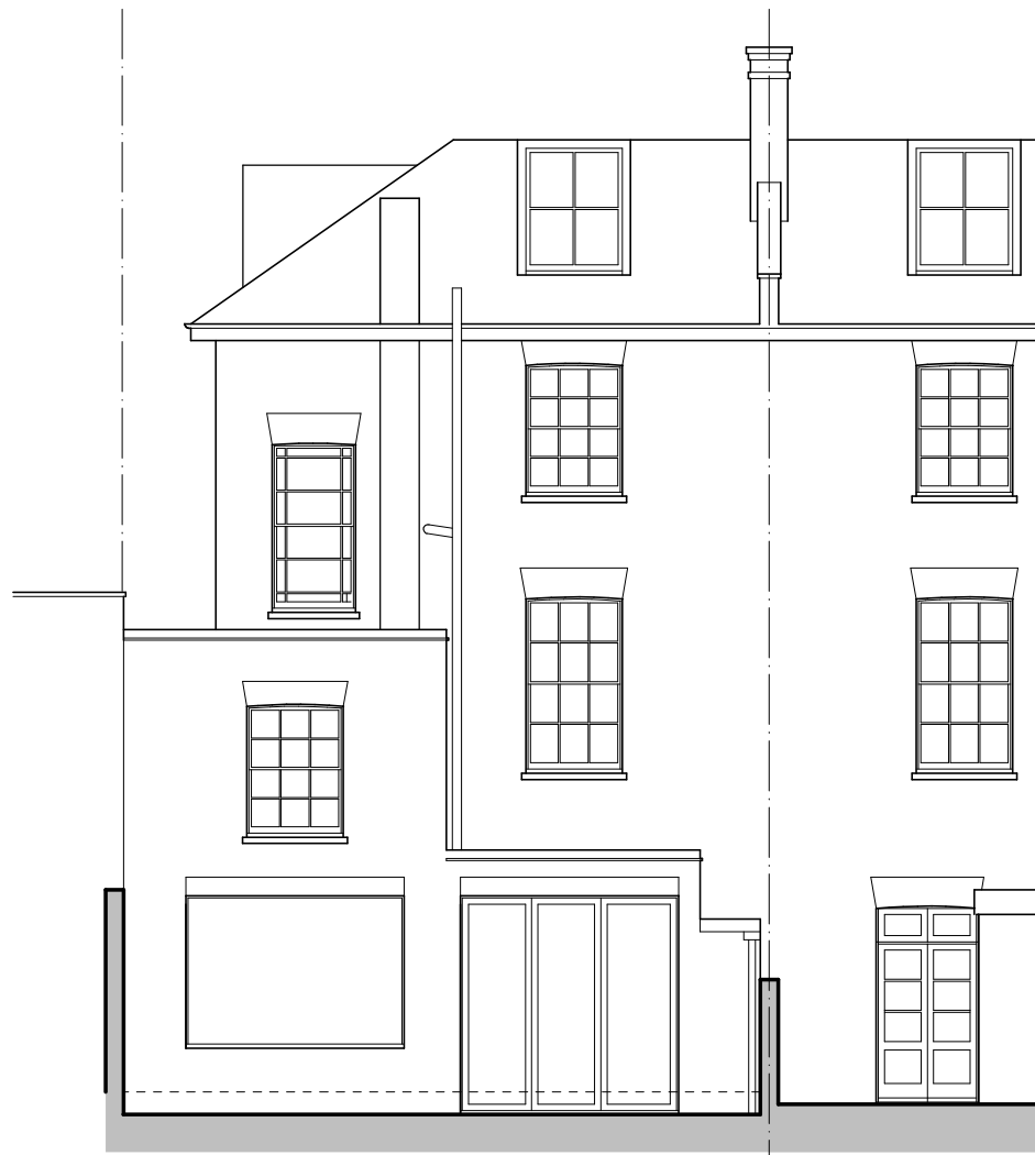
REAR ELEVATION AS PROPOSED brickwork and timber-framed glazed doors and window; 1st floor window to match existing
