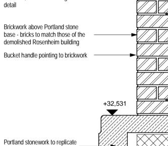
original stone facade 215mm blockwork wall laid on flat Steelwork to support new facade to structural eng's detail
