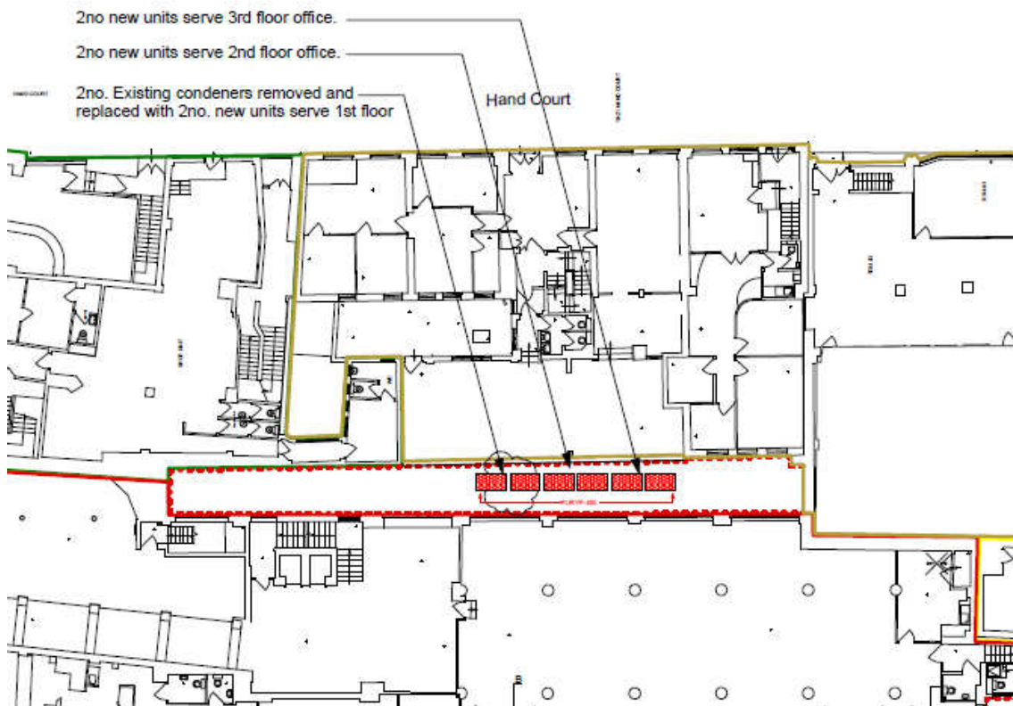
The landlord’s layout of external condenser units.
