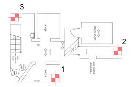
DENOTES TRIAL PIT TO DETERMINE BASE DEPTH/PRO-JECTION OF WALL/FOOTING AND CONFIRM GROUND CON-DITIONS. ASSUME 1m x 1m by 1m DEEP.
