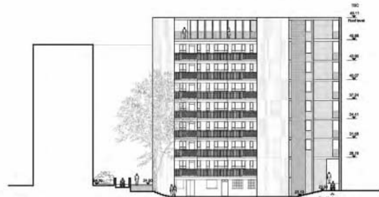
West rear elevation showing extension & changes to cladding
