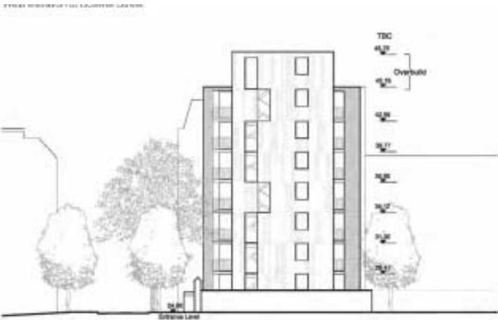
South elevation showing end wall of extension
