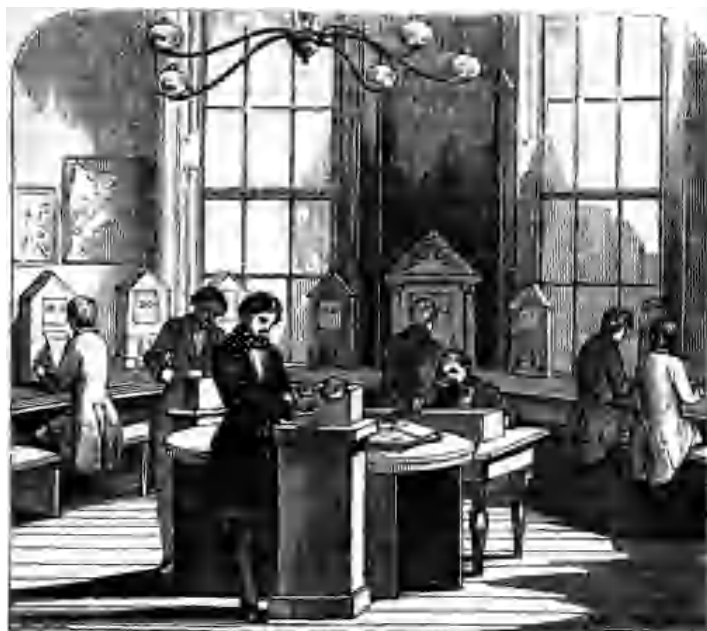
The Instrument Room at Charing Cross A Bain printing telegraph in the foreground The room is circular, in one of Nash's famous "pepper-pots"
