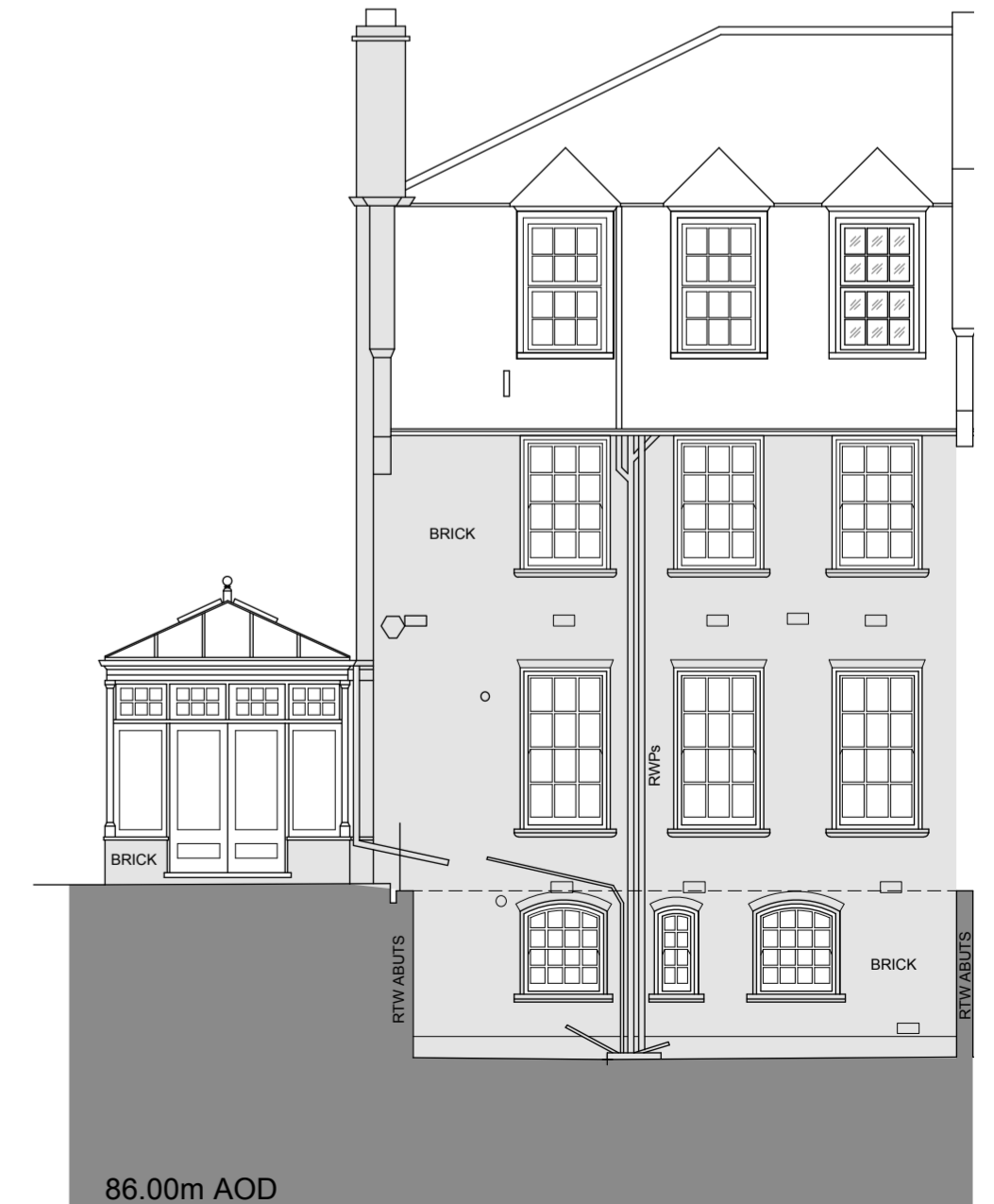
SOUTH WEST ELEVATION
