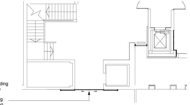
The proposed Bi-Parting sliding door is to be repositioned in the lobby and will improve peak pedestrian flows during opening hours of the building.
