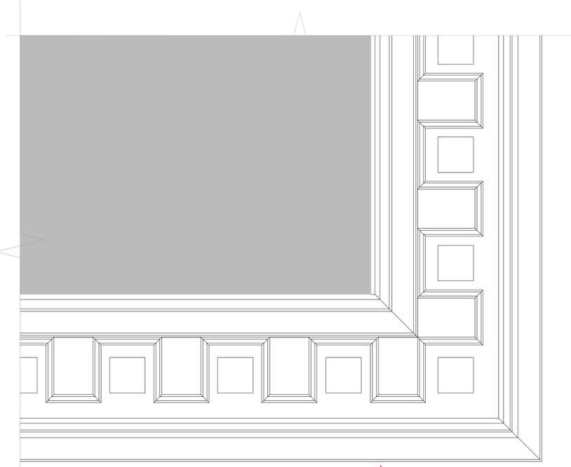
**PART REFLECTED EAVES SOFFIT PLAN
