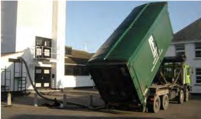
Figure 11: Biomass delivery truck pumping wood fuel into a storage facility
