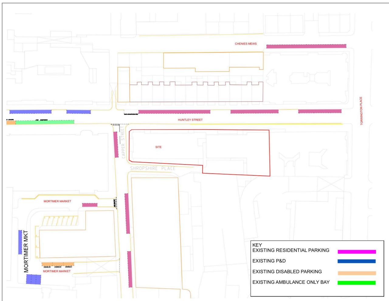
Figure 3.5: Existing Parking Controls Surrounding Site
