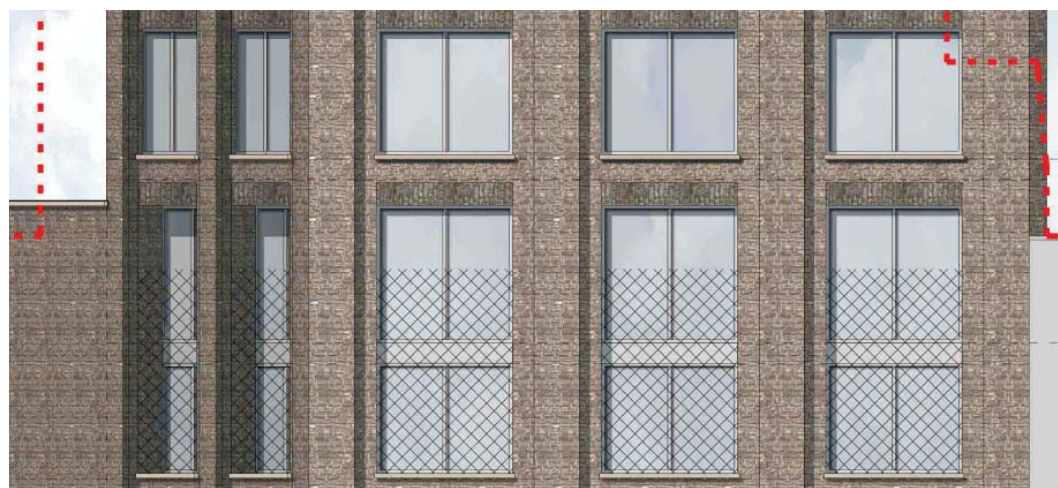
North elevation showing ground floor security fencing to commercial windows
