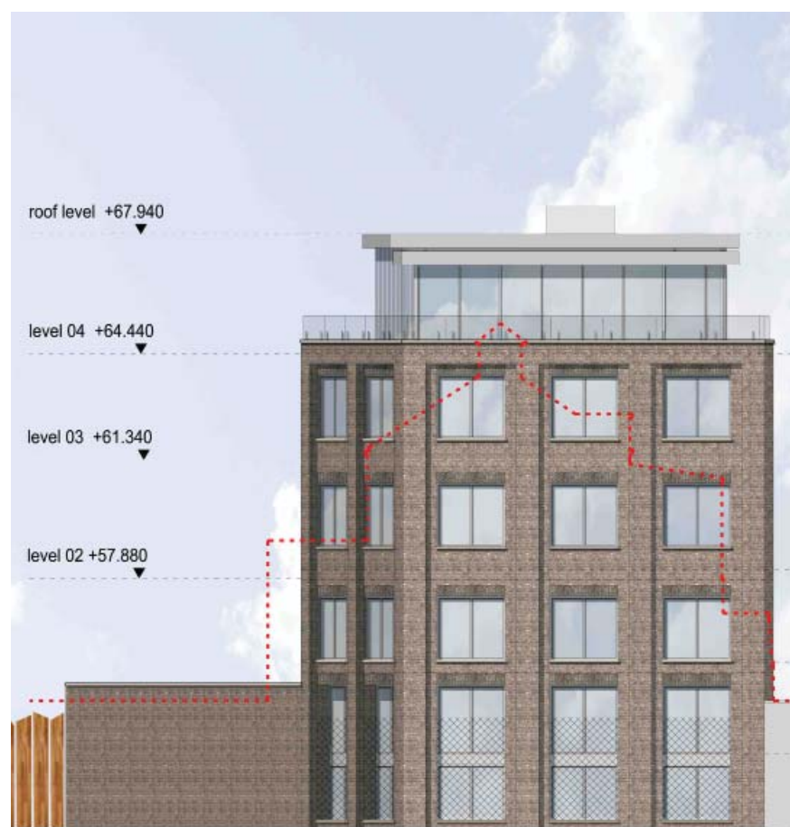
North facing elevation of 25 Ferdinand Street
