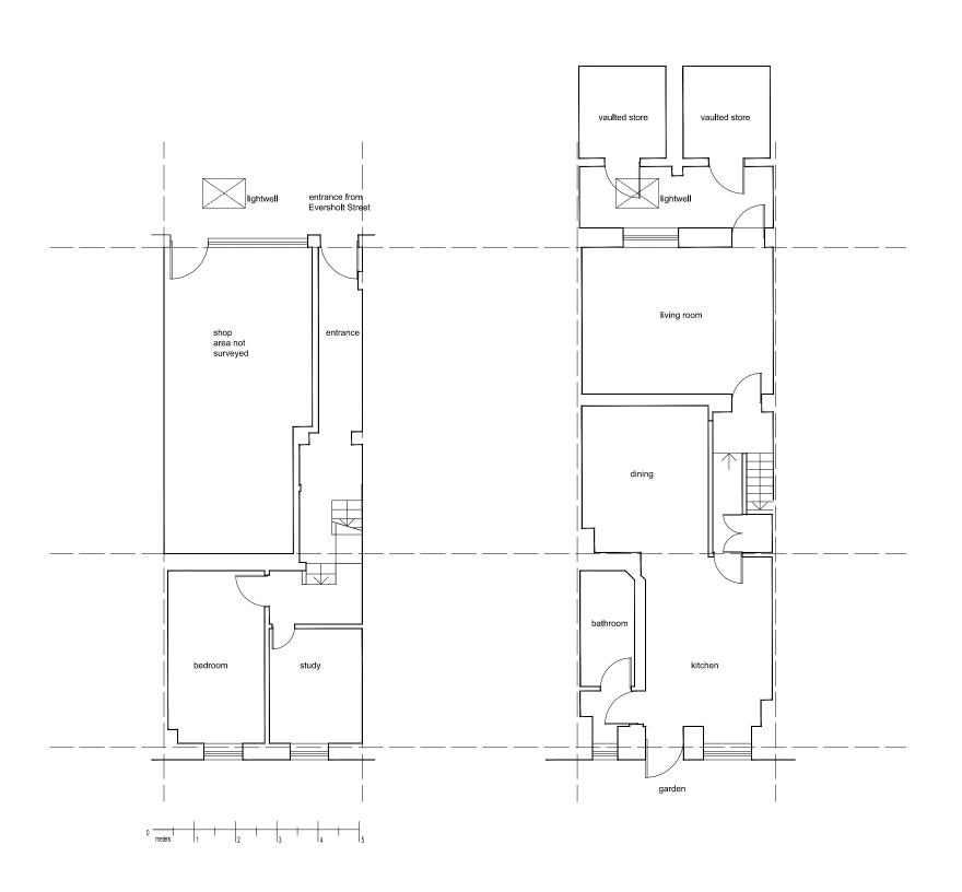
pre existing ground floor plan scale 1:100 pre existing basement floor plan
