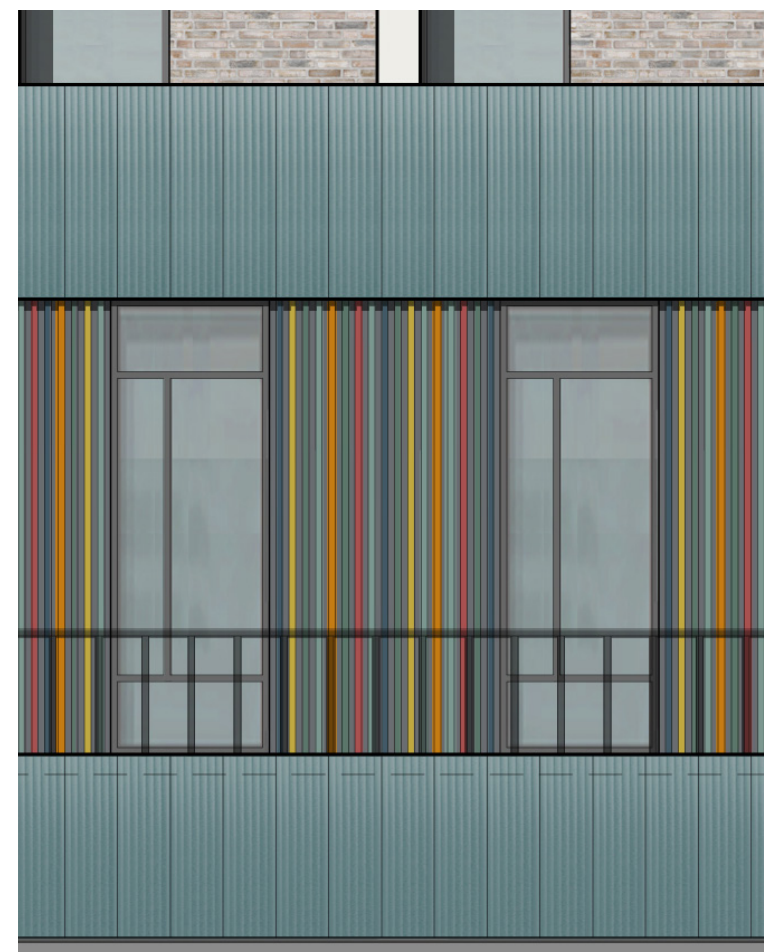
Detail of fluted ceramic panels and baguettes showing indicative colour palette
