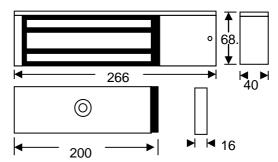
The EM20DS series lock is a surface mount single "face to face" electro-magnetic lock offering up to 1200lb of holding force these locks can be used on either out-swing or inward opening doors.
