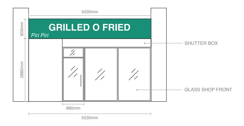
MATERIAL USED: Flat painted signage Grilled O Fried, Piri Piri 1 main door (980mm) with a full glass shop front NAME: Existing shop front and signage SCALE: 1:50 on A4 DATE: 17.11.2014 DRAWING NO: 221-01
