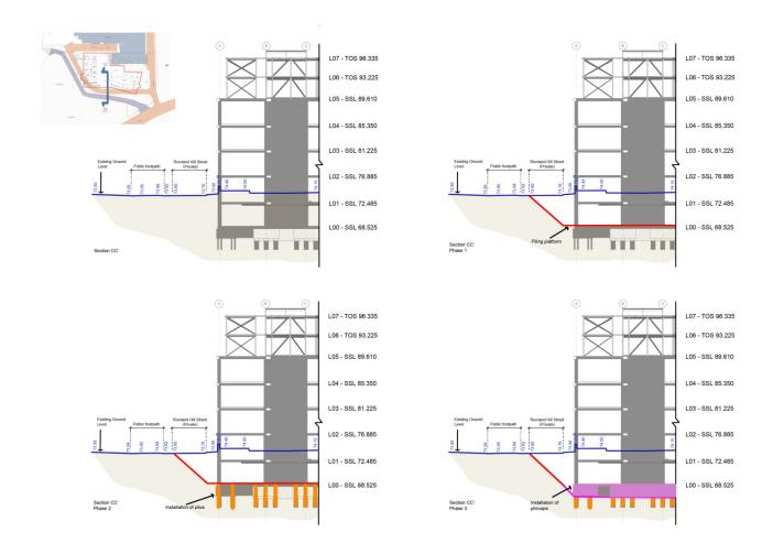
The image above shows the short section West/East through the building noting the different levels at the various stages. Note the proposed batter back of the slope along the public footpath. This is subject to site conditions and to closing the path of to pedestrians. Piled temporary works could also be used along the west section of the building noting that the slope drops down towards the North. This might require a piling platform that is formed in terraces.
