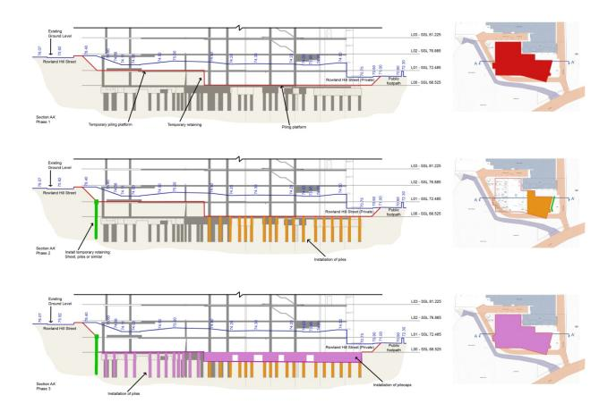
The image above shows the long section North/South through the building noting the different levels at the various stages. Note the proposed location of the temporary piling platform and the location of the temporary piling.
