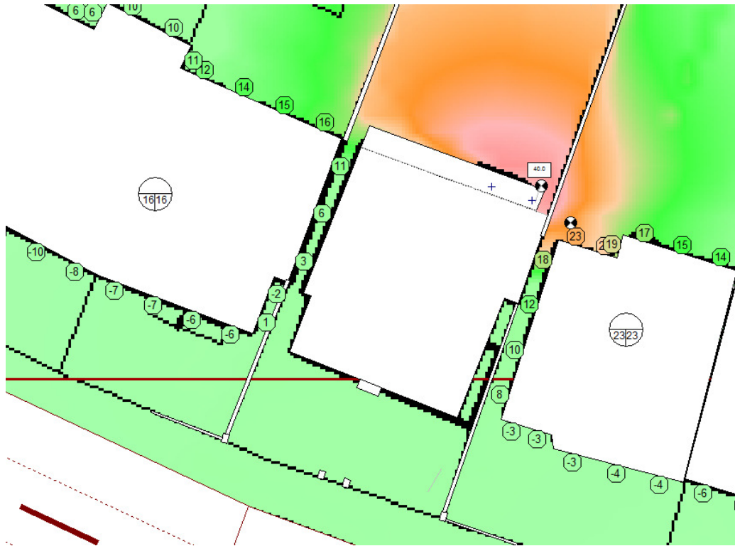
Fig 1: plan view of area local to the proposed plant including noise mitigation measures
