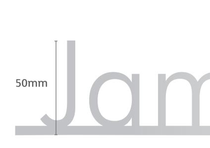
Tenant names in 3mm thick brushed stainless steel Minimum stroke width needs to be 4mm to allow for a 3mm joint between stray dots from letter 'i'
