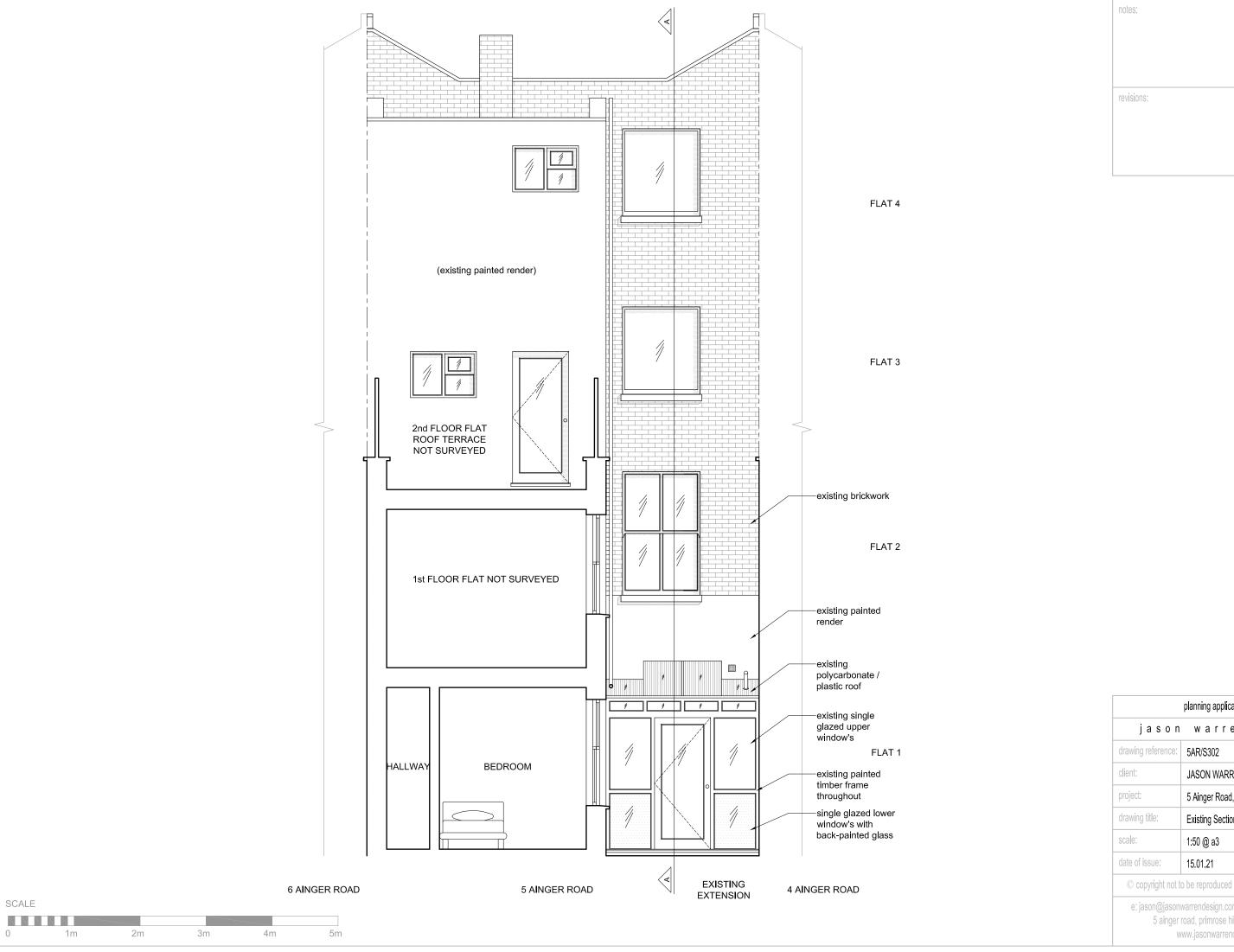
planning application issue jason warren design JASON WARREN 5 Ainger Road, Ground Floor Flat Existing Section B-B
