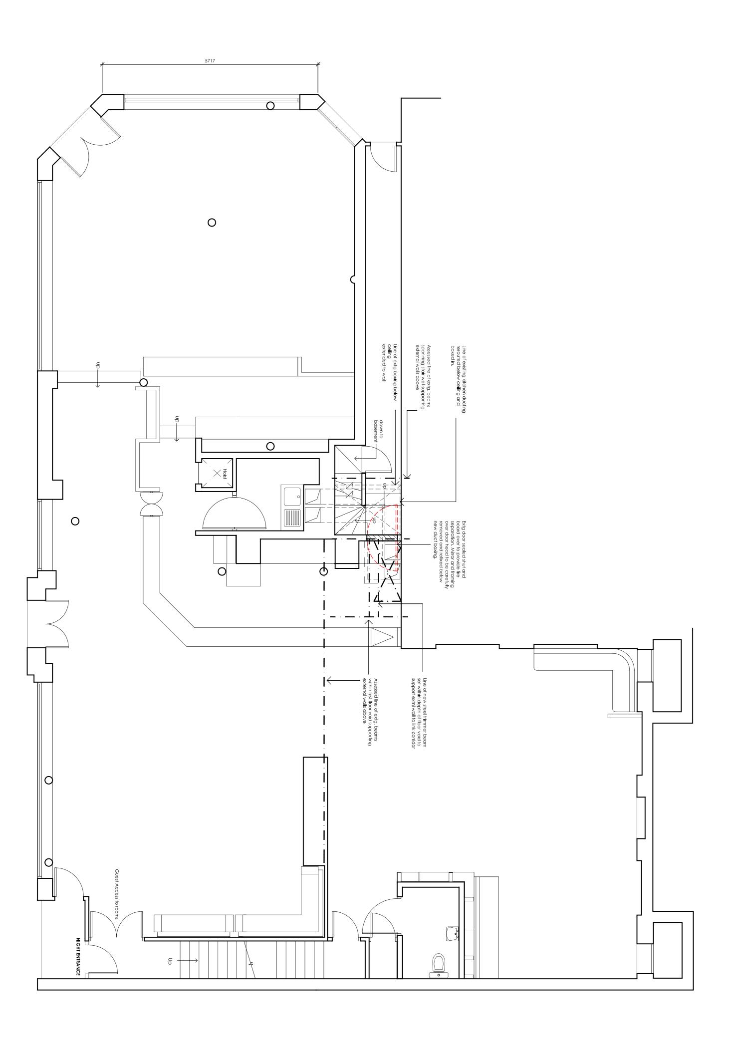
B Beams support to new lift indicated
