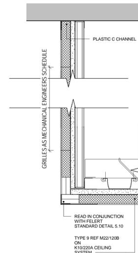
10 TYPE 9 BULKHEAD ACCESS PANEL DETAIL
