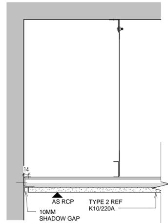
5 TYPE 2 PERPENDICULAR PERIMETER DETAIL
