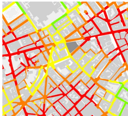
Public transport attraction Volume distance decay from TCR, Holborn, Covent Garden Stations PM Peak R 2 percentage = 11%
