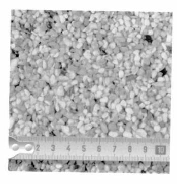
The image to the left is indicative of the Pearl Quartz 2-5mm Resin Bonded Aggregate to be applied to the front driveway.
