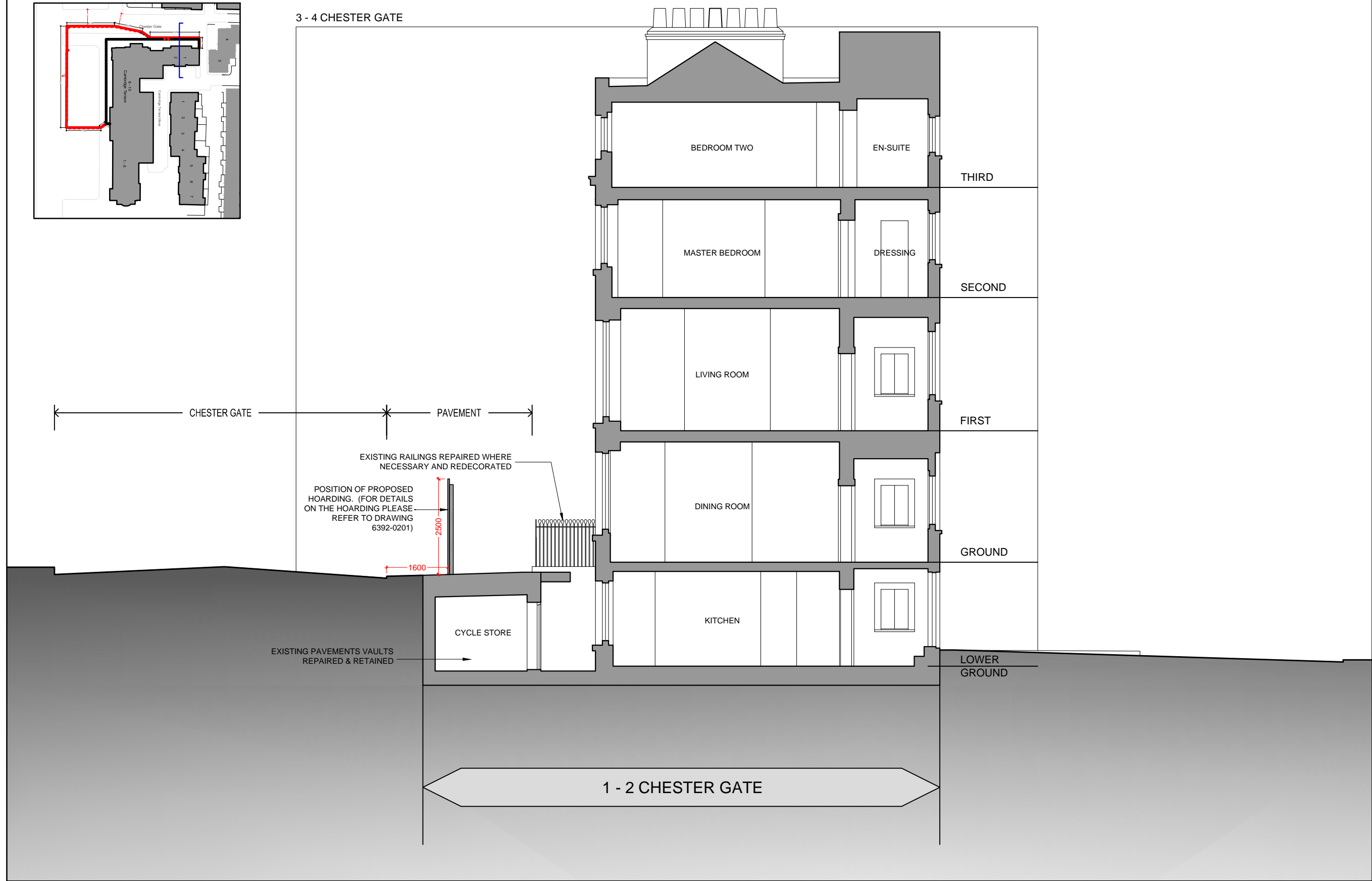
SITE SECTION SHOWING HOARDING BOARD IN RELATION TO THE FACADE OF CHESTER GATE
