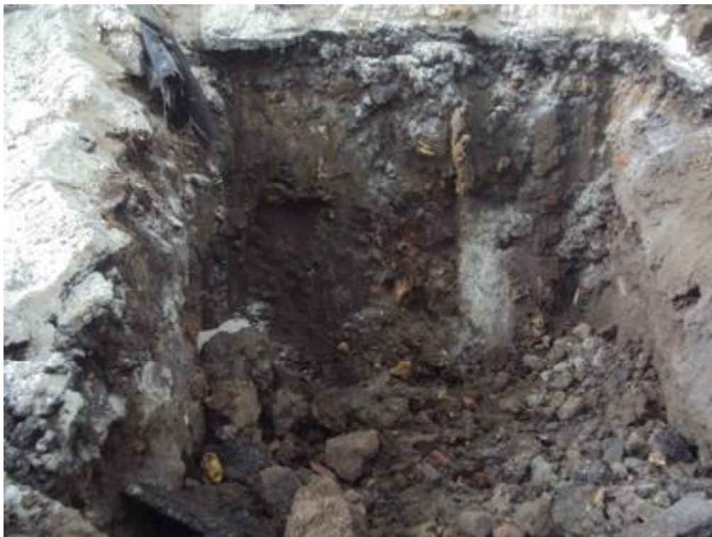
Photograph 8: TP3 – Made ground profile
