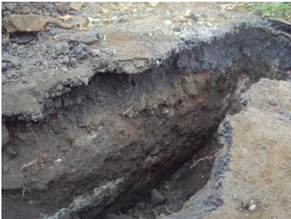
Photograph 2: TP1 – Fine surface roots and made ground below surface layer
