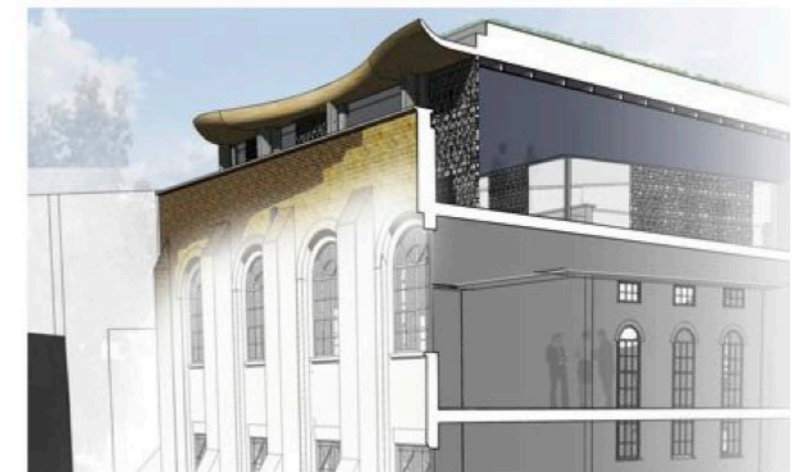
3d cad model study looking at a possible shape of the eaves of the roof and materiality of the new terrace at an early design stage.
