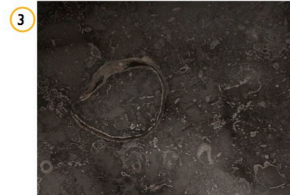
dark coloured natural British stone with fossilised veining to the solid panels between glazed areas.
