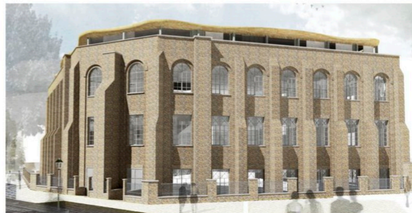
3d cad model study looking at a possible shape of the eaves of the new roof and reducing its impact in relation to the existing building as seen from Peto Place.
