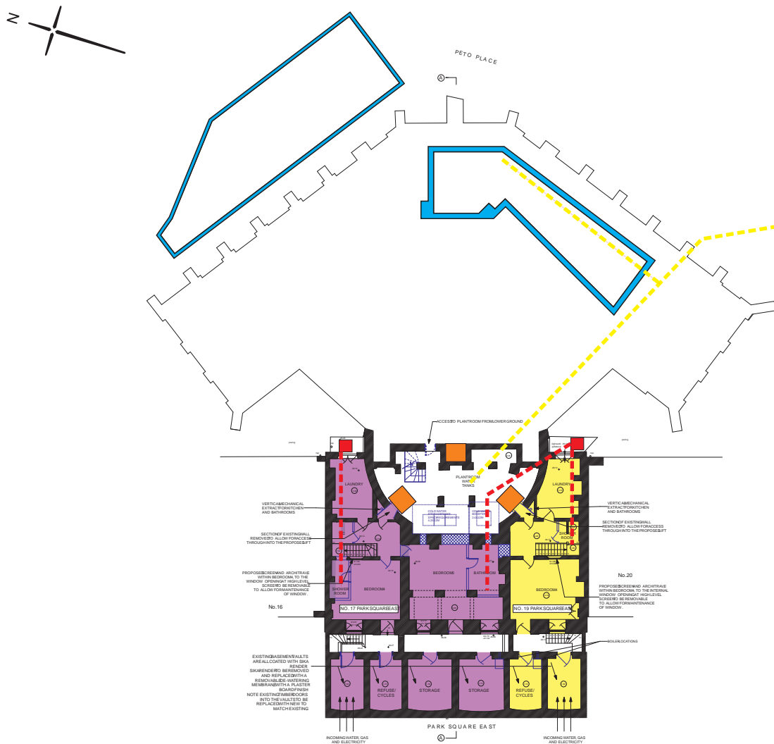
Fig 17 Plan of proposed basement level (HUB Architects and Designers Dwg. No. 1126-PL-01 Rev. K 12/07/2014)
