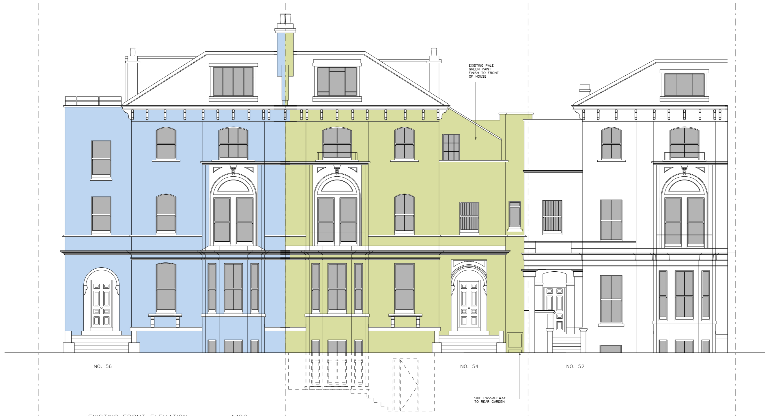
1 EXISTING FRONT ELEVATION 1:100
