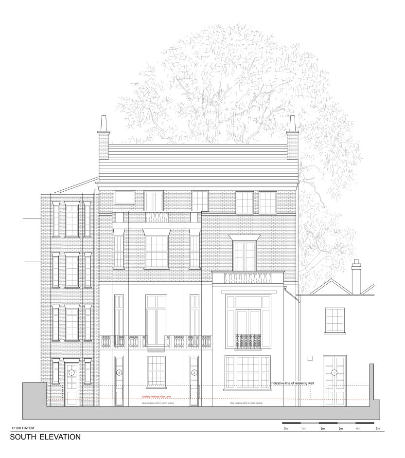
Form new painted hardwood single glazed doors and frames with lambs tongue moulding to match or extend existing frames
