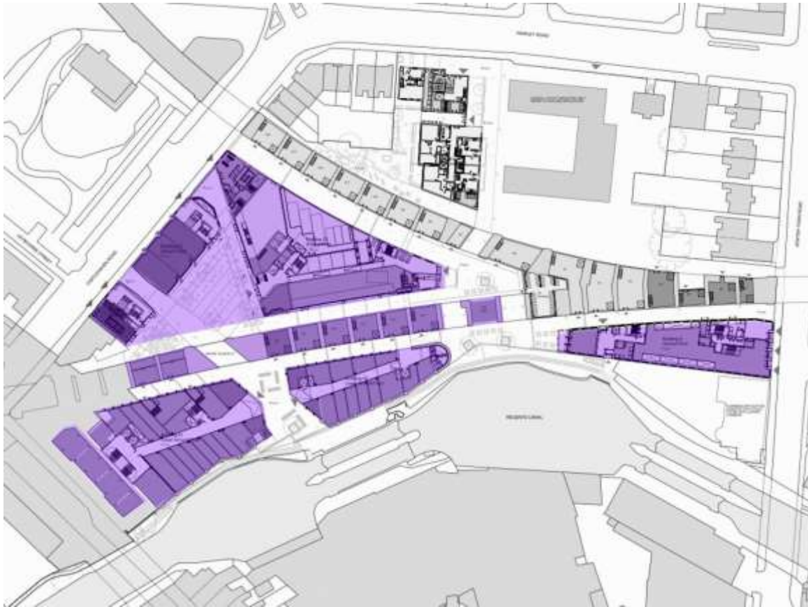
Fig.4: Plan of the application area with proposed single / upper basements highlighted. The northernmost triangular shaped area will have a secondary basement below, but its' location is not deemed archaeologically significant enough to warrant further mitigation
