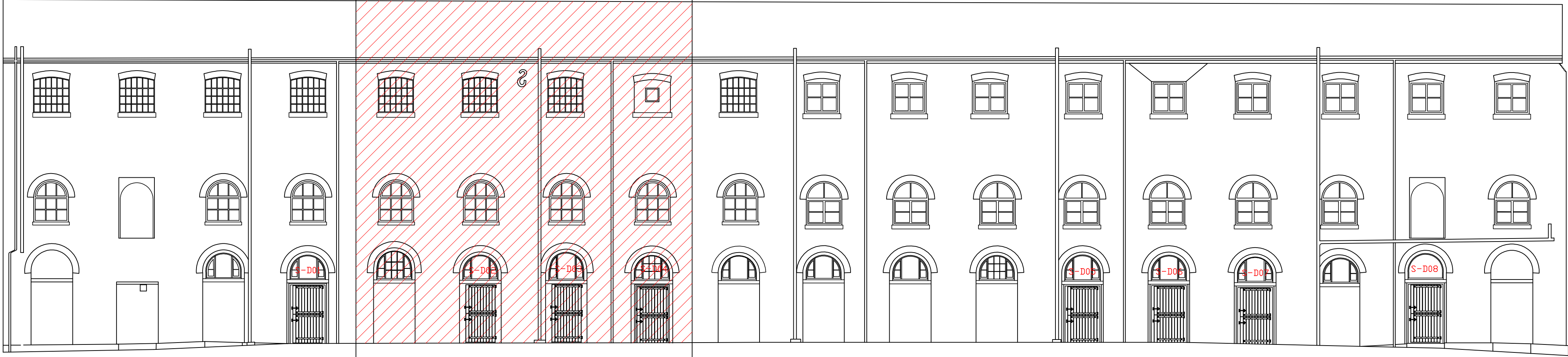
South Elevation as Proposed (Hatched area denotes fire damage)
