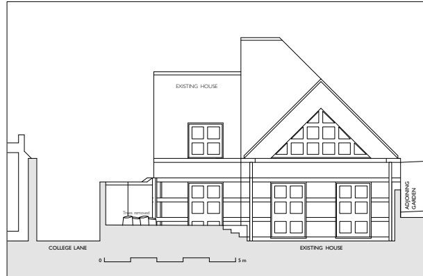
1 : 200 SOUTH ELEVATION TO GARDEN AS EXISTING
