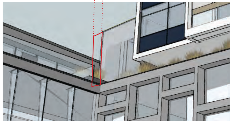
LIFT ENCLOSURE WIDTH REDUCED TO ENSURE CLEARLY DEFINED SEPARATION FROM CPL ROOF
