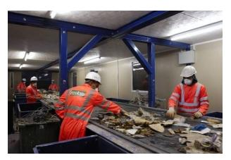
Once the waste has passed a variety of sieves, magnets and other processes it then passes through hand segregation units to maximise recycling.
