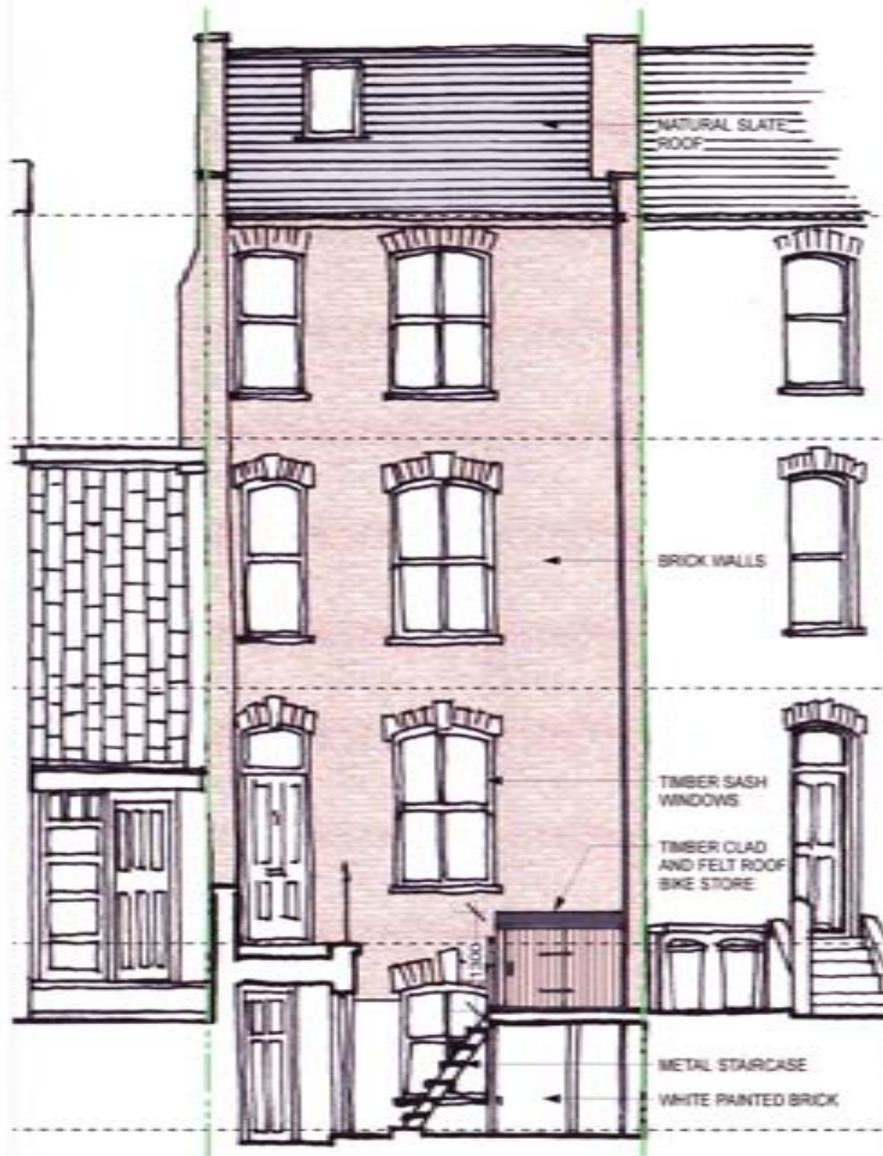
PROPOSED FRONT ELEVATION @ SCALE 1:100
